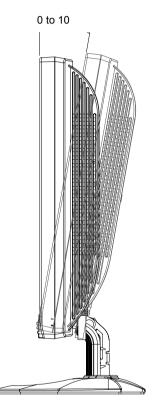
Figure 1-4: Tilting the Monitor
